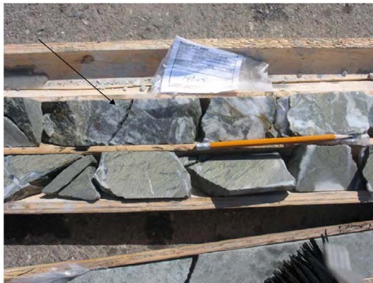
Figure 8.4 Drill Hole DZ06-14 (2) Altered Siltstone with Bedding and Quartz Vein
