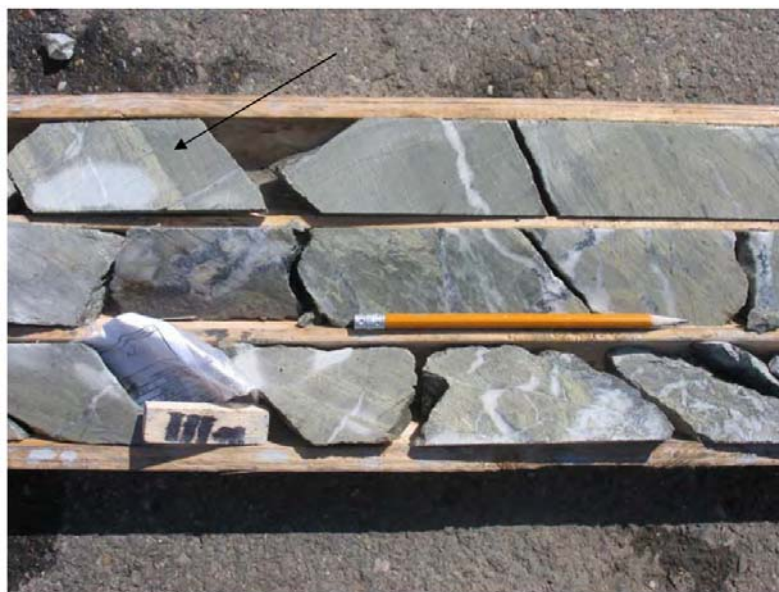
Figure 8.4 Drill Hole DZ06-14 (2) Altered Siltstone with Bedding and Quartz Vein
